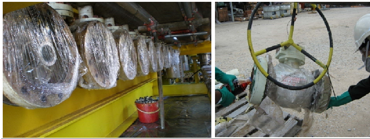
Figure 10 Process equipment covered with plastic wrap
