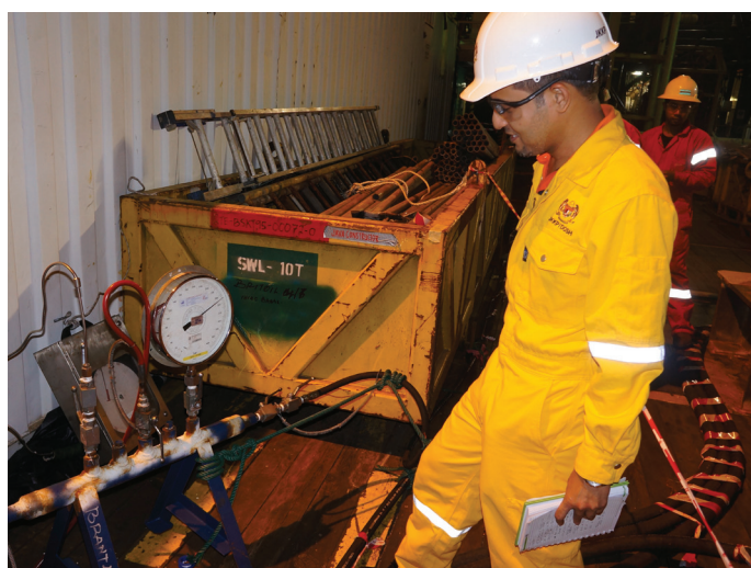
Fasa penahan tekanan ujian hidrostatik pada talian paip dasar laut di atas kapal pemasangan paip milik TL Offshore Sdn Bhd, di luar perairan Terengganu. Holding pressure phase of hydrostatic testing of a sub-sea pipeline on a pipe-laying barge owned by TL Offshore Sdn Bhd, off the coast of Terengganu.
