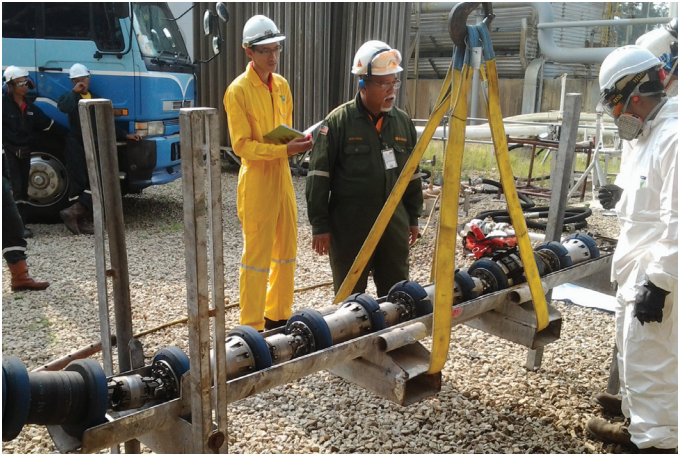
Pemeriksaan penjongkongan pintar dalam operasi terminal eksport di Kemaman. Intelligent pigging inspection at the Export Terminal Operation in Kemaman.
