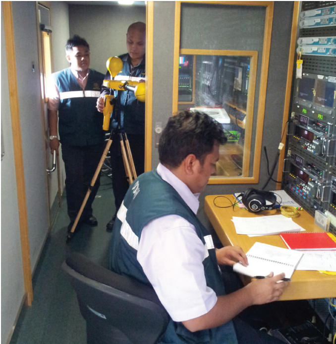
Gambar 7: Pengukuran medan elektromagnet dan medan elektrik diambil di dalam galeri di atas kenderaan. Photo 7: Electromagnetic field (EMF) and electric field (RF) levels were measured in the On-board Vehicle Gallery.
