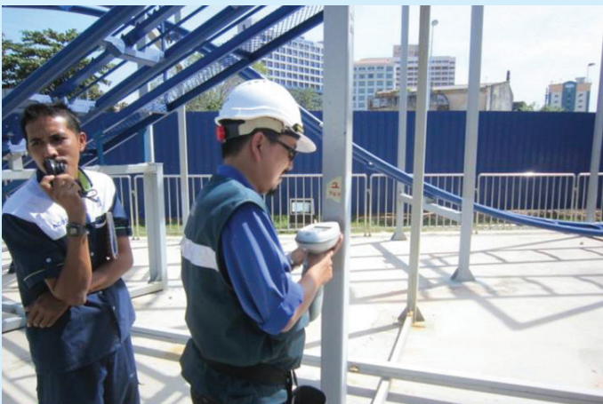
Gambar 13: Ujian ke atas bahan pada roller coaster menggunakan kaedah Positive Material Identification (PMI). Photo 13: Applying Positive Material Identification (PMI) method in a material test for roller coaster structures.
