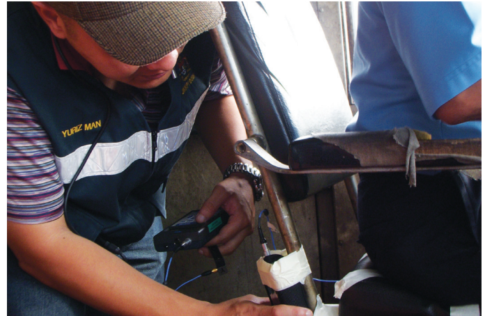
Gambar 10: Getaran whole body dihantar melalui kerusi atau kaki pekerja yang memandu keretapi lokomotif. Photo 10: The whole body vibration (WBV) is transmitted through the seat or feet of the employees driving the locomotive.
