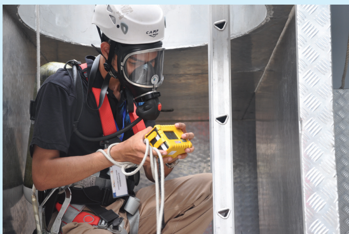
Gambar 1: Alat penguji gas digunakan semasa latihan praktikal. Photo 1: The multi-gas detector being used during practical training.
