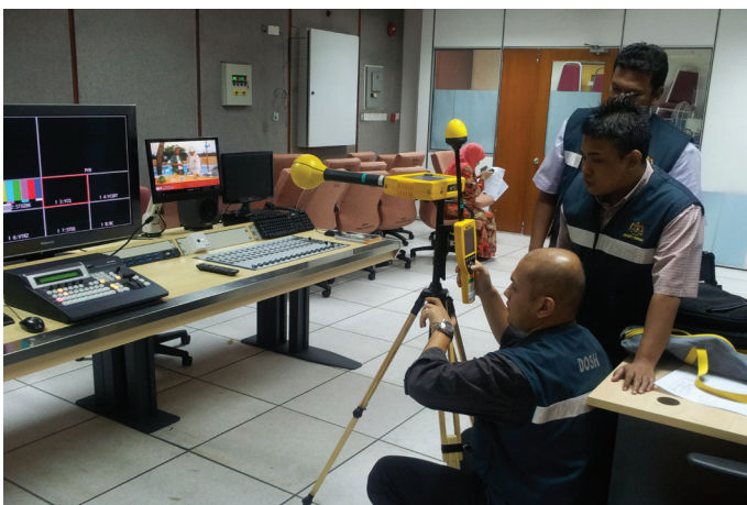
Gambar 5: Pengukuran sinaran tak mengion dijalankan di Bilik Konti. Photo 5: Non-Ionising radiation is being measured in the Conty Room.
