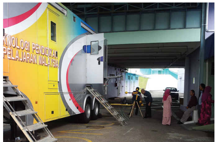
Gambar 6: Bacaan medan elektromagnet dan medan elektrik sedang diambil pada penerima dan pemancar di atas kenderaan. Photo 6: Electromagnetic field (EMF) and electric field (RF) readings were being taken at the receiver and transmitter (on-board vehicle).
