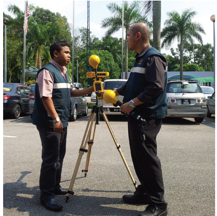
Gambar 8: Pengukuran medan elektromagnet dan medan elektrik turut diambil pada penerima (persekitaran luar) menggunakan selective radiation meter dan meter medan jalur lebar. Photo 8: Electromagnetic field (EMF) and electric field (RF) levels were also measured at the receiver (external environment) using the selective radiation meter and the broadband field meter.
