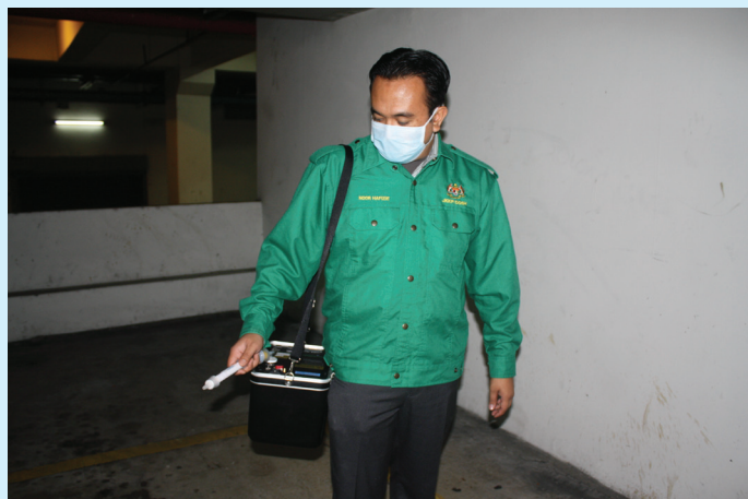
Pengukuran gas radon di ruang parkir menggunakan kaedah sniff. Measuring radon gas level in a car parking area using the sniff method.
